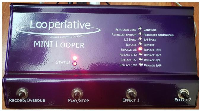
The top of the LP2 has 4 buttons and 10 LEDs. The two LEDs next to the word "STATUS" are used to indicate basic status of tracks 1 and 2. The top LED is for track 1 and the bottom LED is for track 2. The 8 LEDs on the side are used to select different effects for the two effect buttons and are used for additional status. The 4 buttons are multipurpose depending on the mode. Their meaning in normal mode is printed under each button.
